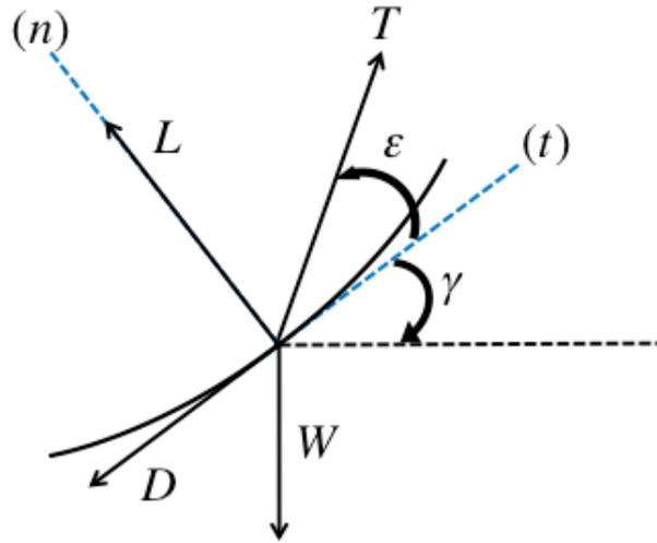
Figure 14: Symmetric flight within a vertical plane
