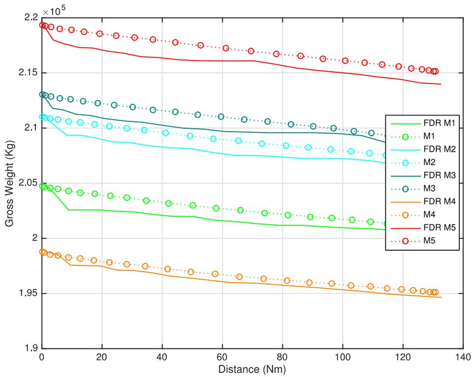
Figure 23: Gross Weights comparison between conventional (real) and CCO (optimized) flight data for several mass scenarios as a function of Distance.
