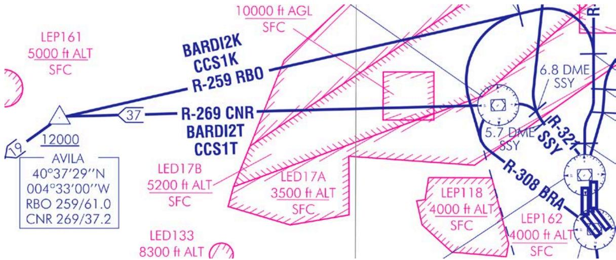
Figure 17: SIDs RWY 36L: Detailed view of selected flight segments associated to BARDI2T/ CCS1T & BARDI2K/CCS1K SIDs
