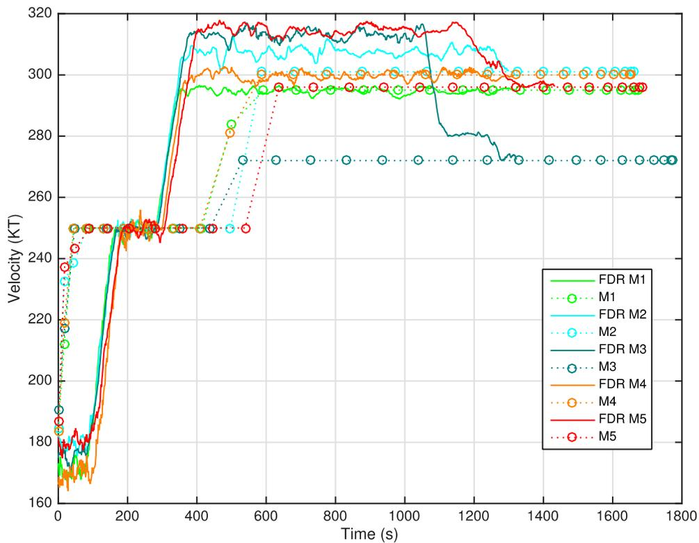
Figure 28: Velocity comparison between conventional (real) and CCO (optimized) flight data for several mass scenarios as a function of time.
