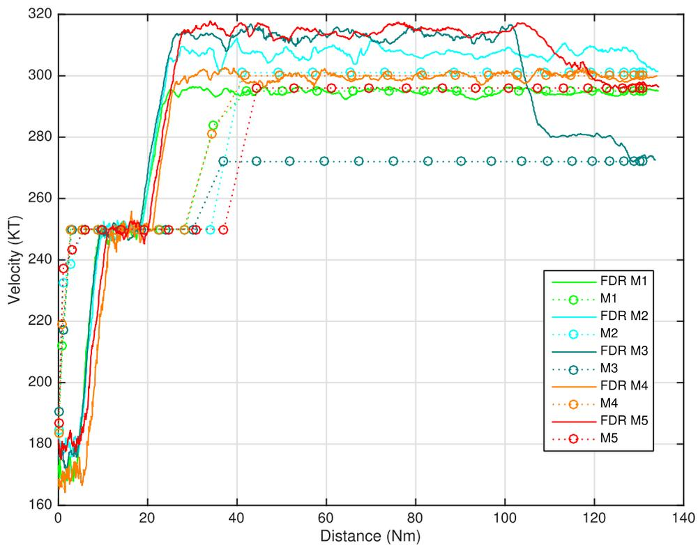
Figure 27: Velocity comparison between conventional (real) and CCO (optimized) flight data for several mass scenarios as a function of distance.
