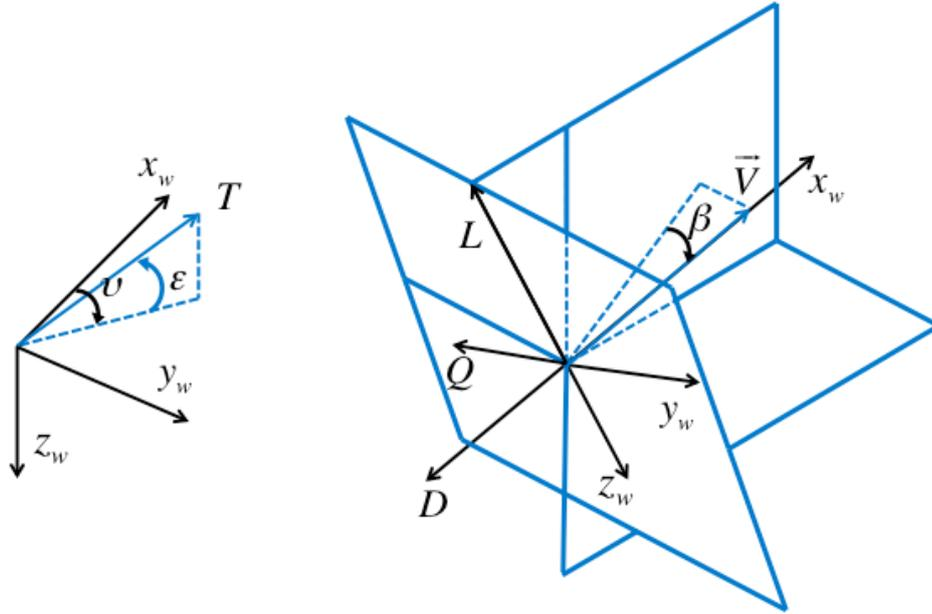
Figure 13: Wind axes system & thrust orientation
