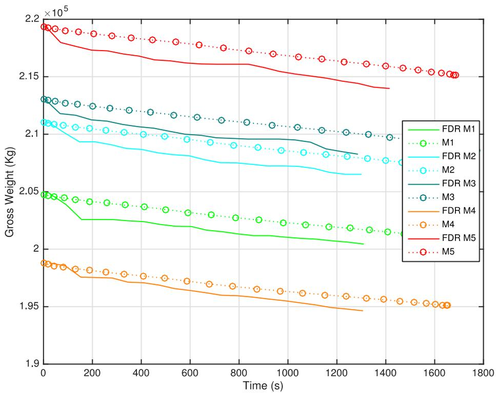
Figure 24: Gross Weights comparison between conventional (real) and CCO (optimized) flight data for several mass scenarios as a function of Time.
