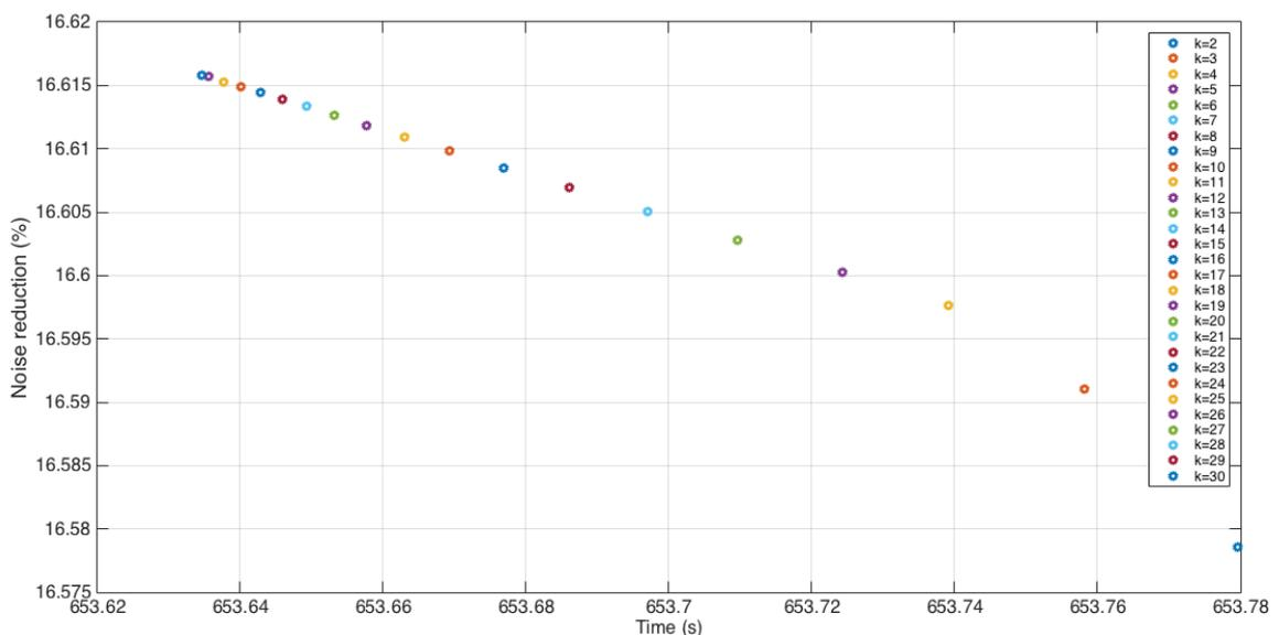
Figure 19: Conventional departure compared to Optimized CCO – Noise reduction (%) vs Time (s)
