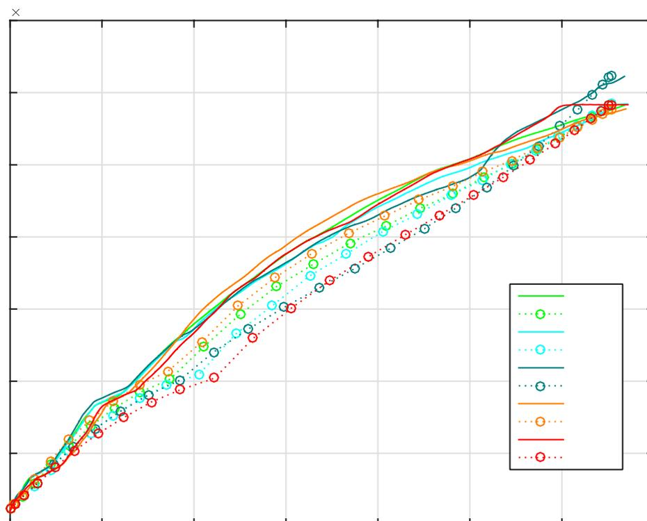
Figure 21: Vertical profile comparison between conventional (real) and CCO (optimized) flight data for several mass scenarios, as a function of distance
