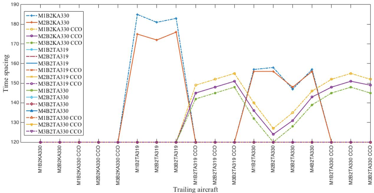
Figure 31: Time separations between aircraft operating BARDI2T/ CCS1T & BARDI2K/CCS1K SIDs.
