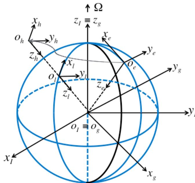
Figure 9: Reference axes systems
