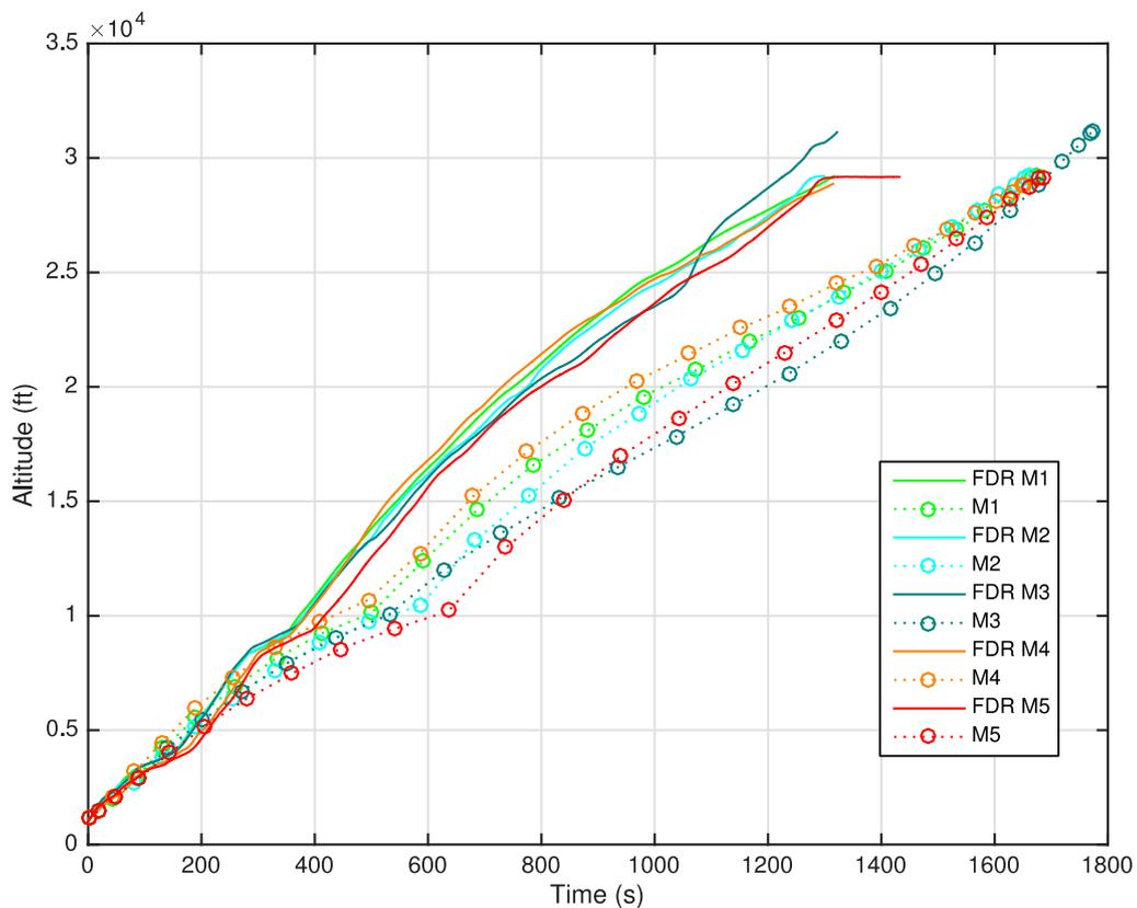
Figure 22: Vertical profile comparison between conventional (real) and CCO (optimized) flight data for several mass scenarios, as a function of time
