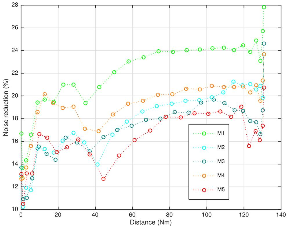
Figure 29: Noise reduction when comparing CCO (optimized) against conventional (real) flight data for several mass scenarios, as a function of Distance (%)
