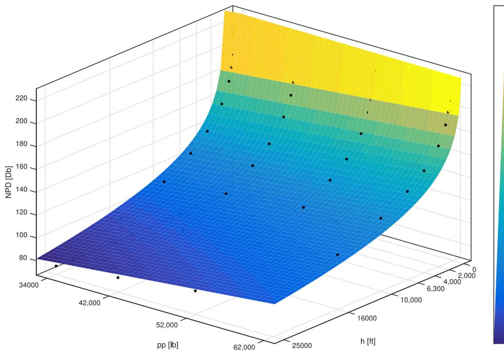
Figure 15: NPD ( $L_{max}$ ) vs engine thrust settings ( $pp$ ), altitude ( $h$ )
