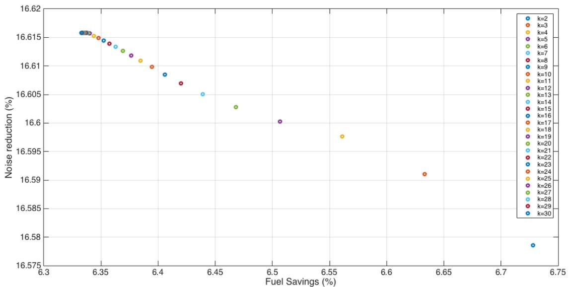
Figure 20: Conventional departure compared to Optimized CCO - Noise Reduction (%) vs. Fuel Savings (%)
