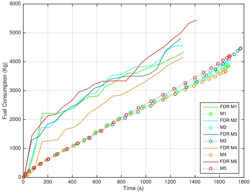
Figure 26: Fuel Consumption comparison between conventional (real) and CCO (optimized) flight data for several mass scenarios as a function of time.
