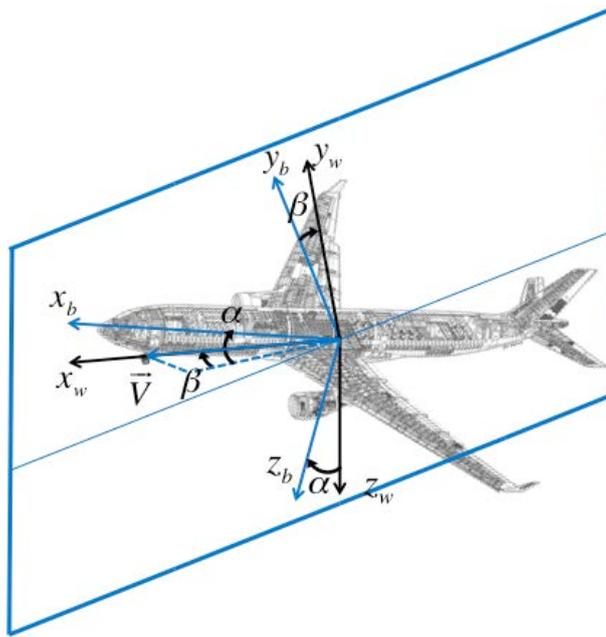
Figure 12: Local body axes system
