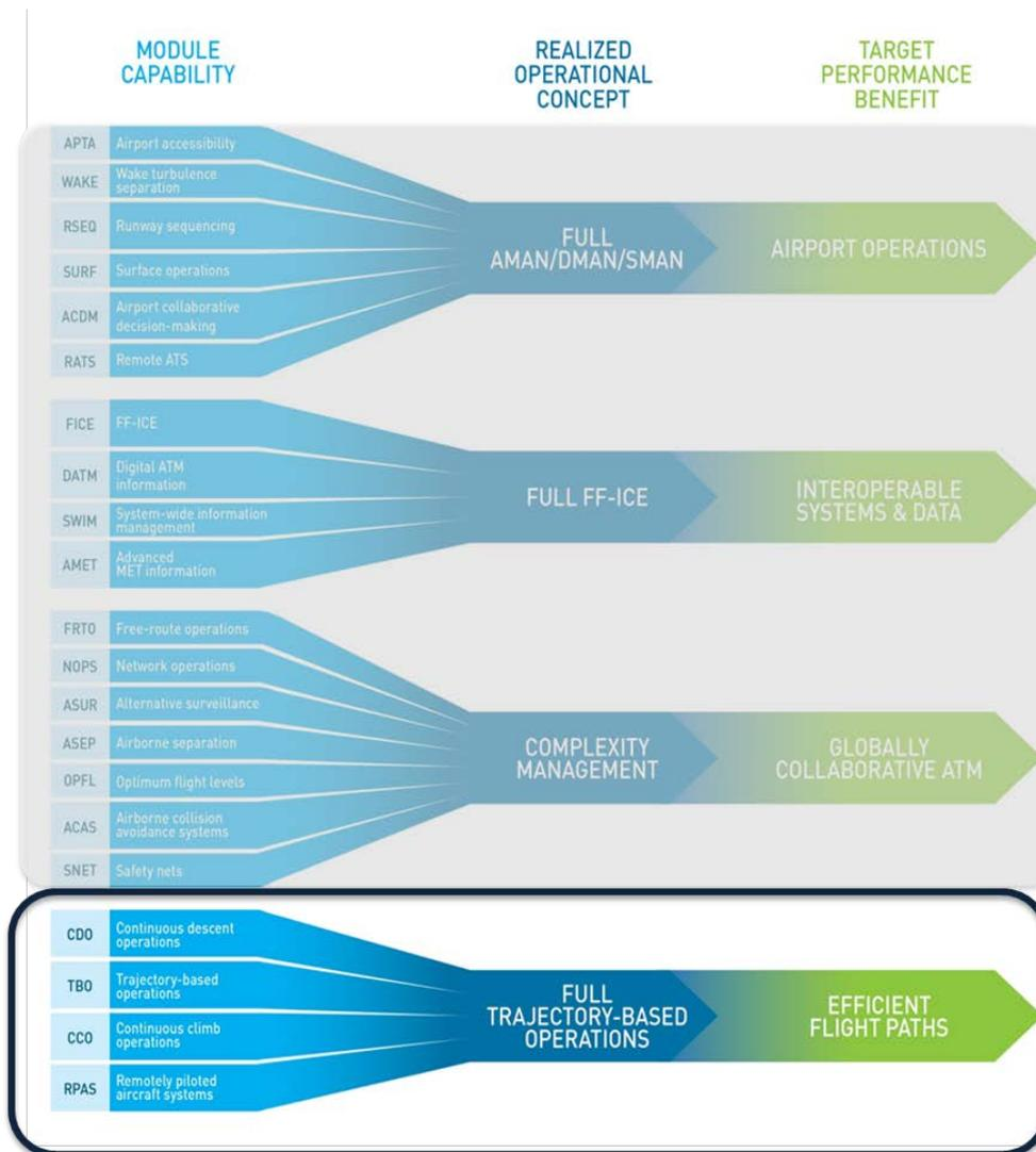
Figure 1: Aviation System Block Upgrades (ASBUs) – Efficient Flight paths
