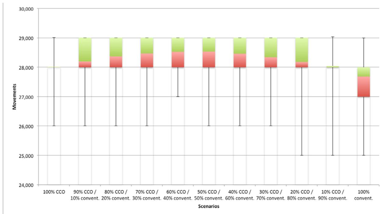
Figure 32: Capacity: Maximum number of aircraft that can be accommodated per hour according to aforementioned scenarios.
