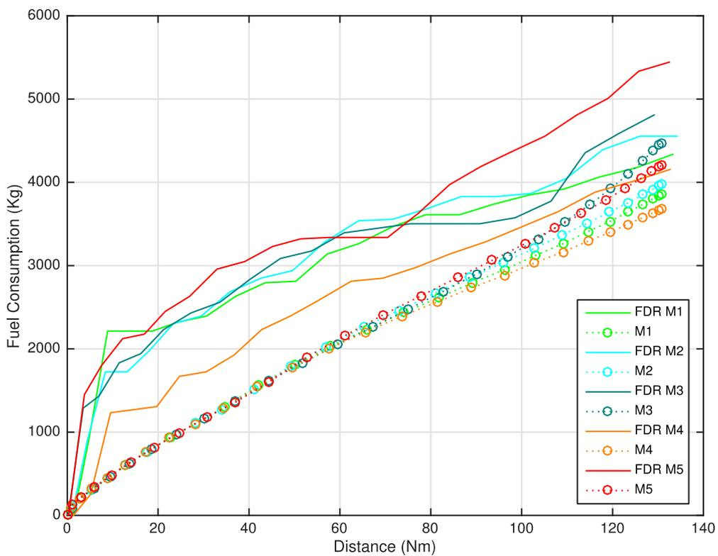
Figure 25: Fuel Consumption comparison between conventional (real) and CCO (optimized) flight data for several mass scenarios as a function of distance.
